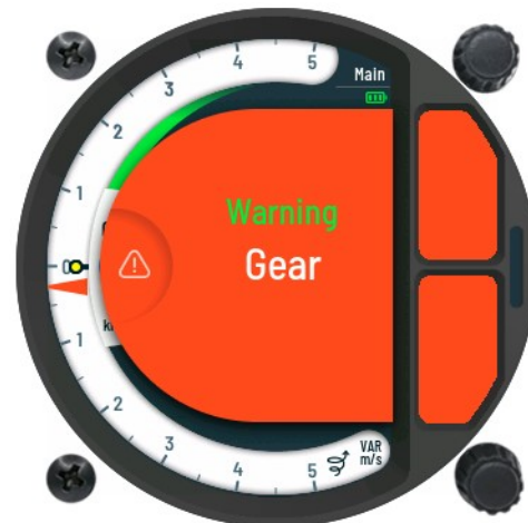
Gear warning view.
